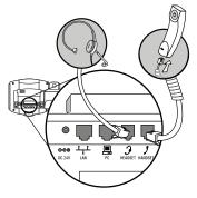
Connect network and power, as shown below. *Note:* Choose either AC Power Option, or PoE (Power over Ethernet).
